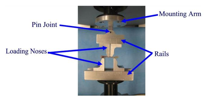
Fig. 13.2. Four-Point Bend Test Fixtures Supporting a Murine Tibia.
