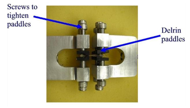
Fig. 13.1. Tensile Test Fixtures Holding a Murine Tibia.
